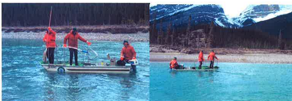
Figure 3.2 Boat-mounted electrofisher used by staff from Alberta Sustainable Resource Development.
