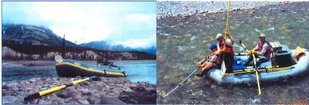
Figure 3.1 Raft-mounted electrofisher used by staff from the Alberta Conservation Association.
