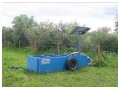
ACA's portable, solar-powered off-channel watering system in use on Bearberry Creek.
