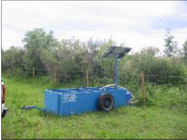
Figure 1. ACA's portable, solar-powered off-channel watering system in use on Bearberry Creek. (Photo: Chad Judd)
