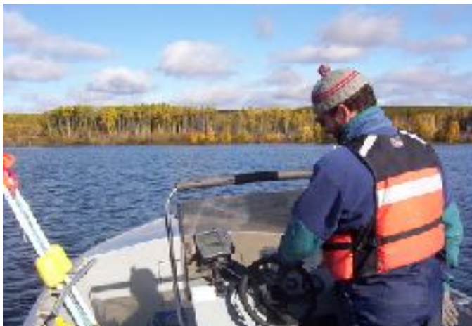
Locating net location using depth sounder and Global Positioning System (GPS) at Ethel Lake. (Photo: Roy Schmelzeisen)
