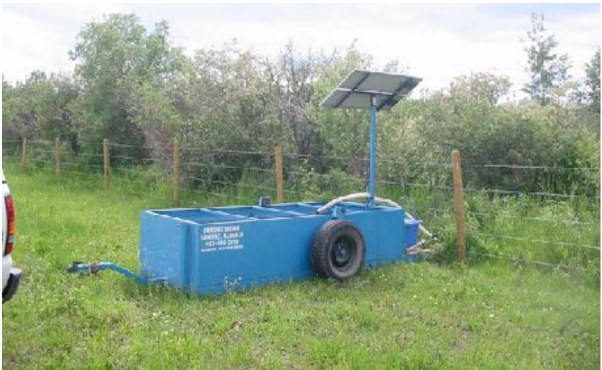
Figure 3. ACA's portable, solar-powered off-channel watering system in use on Bearberry Creek (Photograph by Chad Judd).
