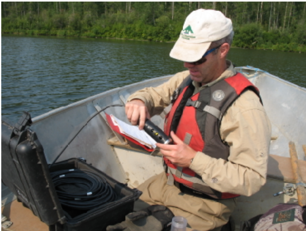
Water quality sampling with YSI unit in Swan Lake. (Photo: Paul Hvenegaard)
