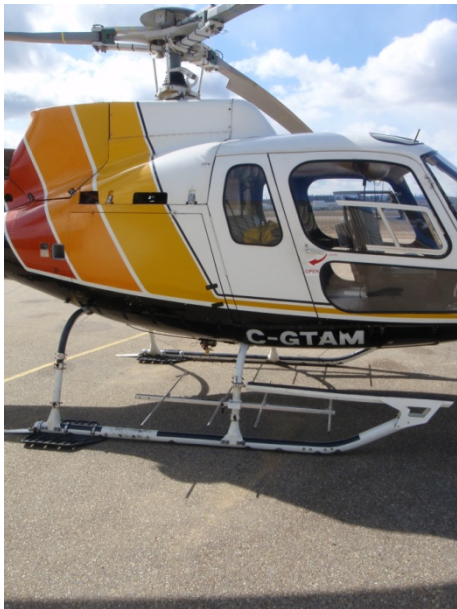
A helicopter fitted with uni-directional Yagi antennae for aerial telemetry surveys. (Photo: Clayton James)
