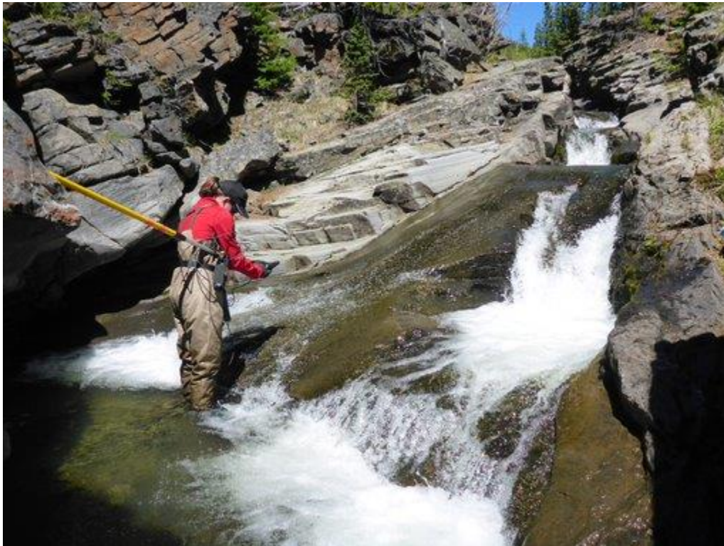
ACA seasonal staff member, Kacey Barrett, adjusts a velocity meter probe below a compound cascade barrier. Photo: Jason Blackburn.
