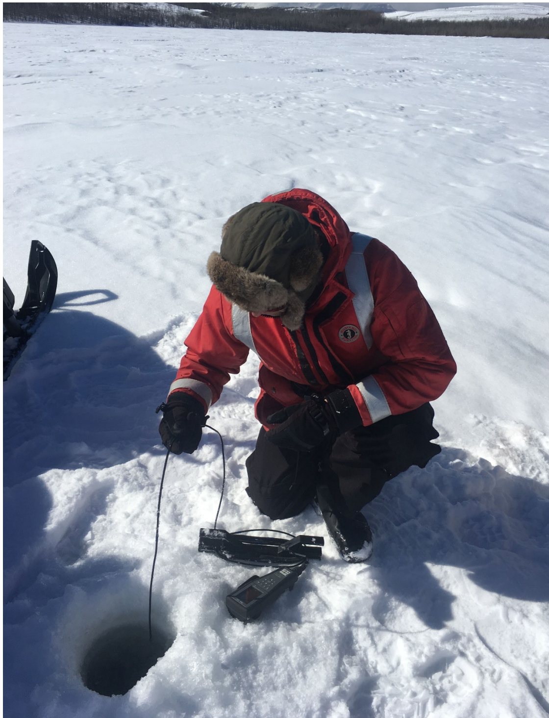
ACA staff measuring dissolved oxygen and water temperature at Bullshead Reservoir in winter.
