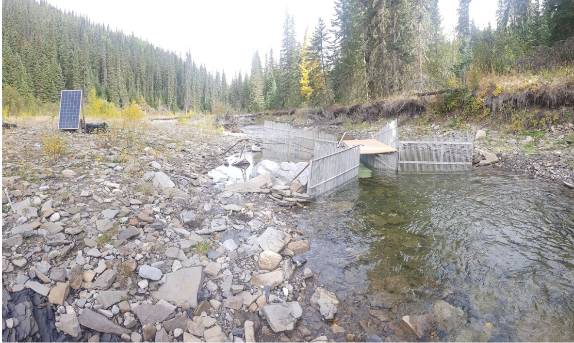
Solar-powered underwater video recording system and fish fence installed in Fall Creek. Photo: Zachary Spence
