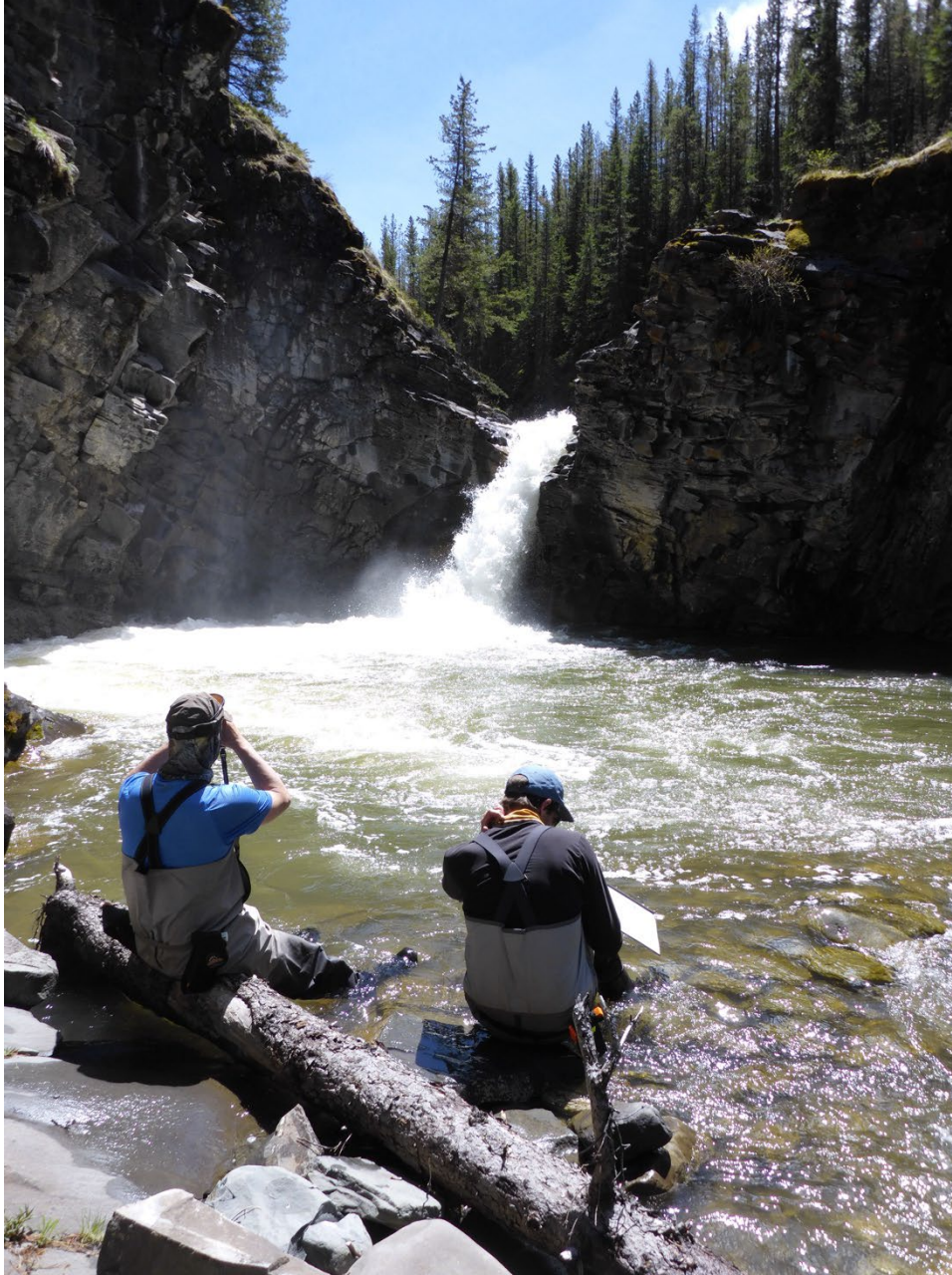
Photo 3. Crew using a laser rangefinder to measure height of a plunge waterfall on Etherington Creek. Photo: Jason Blackburn
