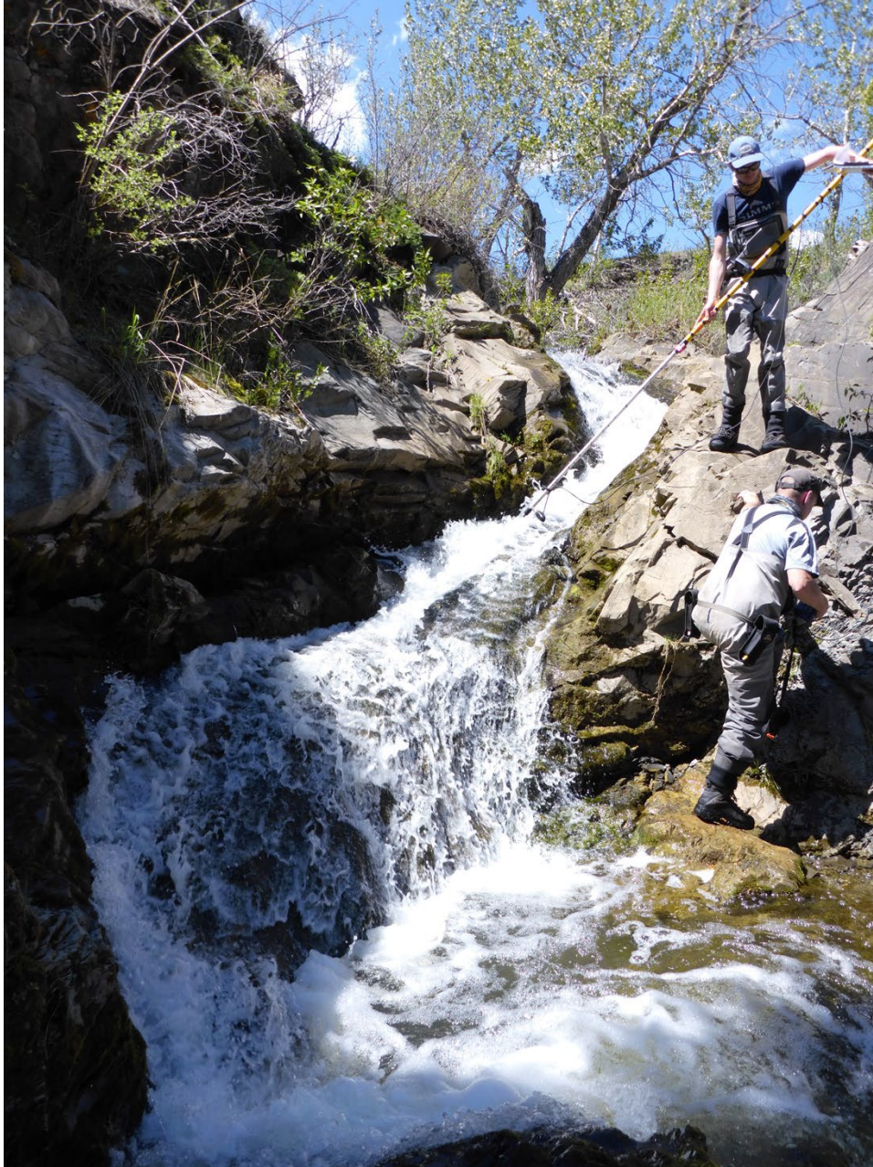
Photo 2. Crew preparing to measure velocity in a chute barrier on Ings Creek. Photo: Jason Blackburn
