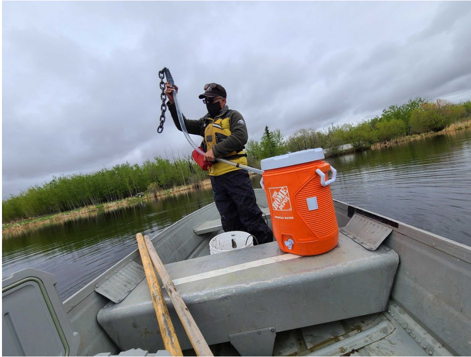
Photo 1. ACA staff using a hose with one-way foot valve to collect composite water sample from Rainbow Park Pond for chemical analysis. Photo: Lindsay Dowbush
