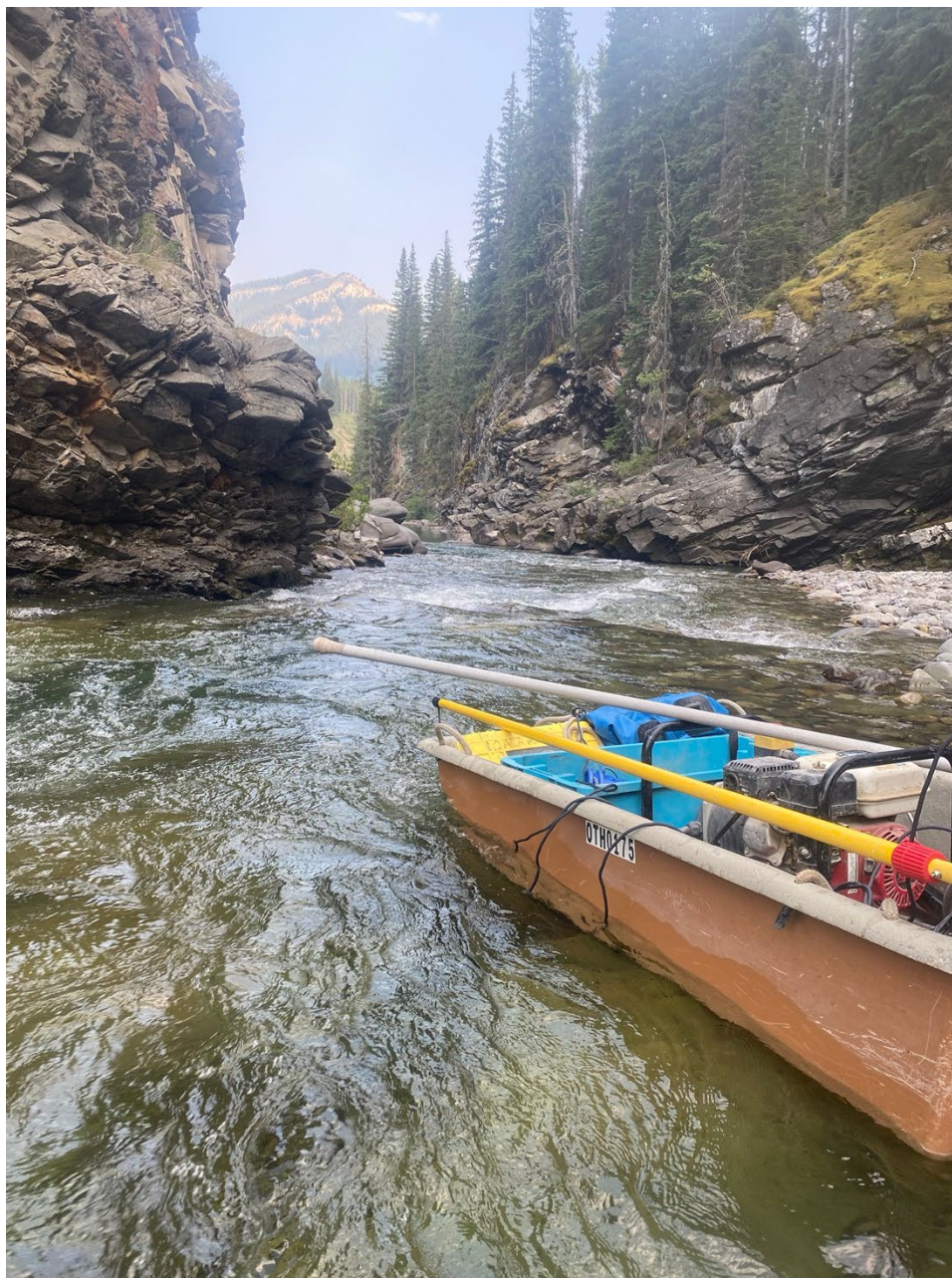
Photo 2. Tote barge electrofishing equipment used on the upper Oldman River. Photo: Brad Hurkett
