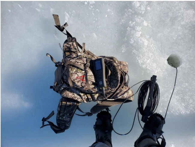
Photo 2. Under ice dissolved oxygen sampling on Shell True North Pond. Photo: David Jackson
