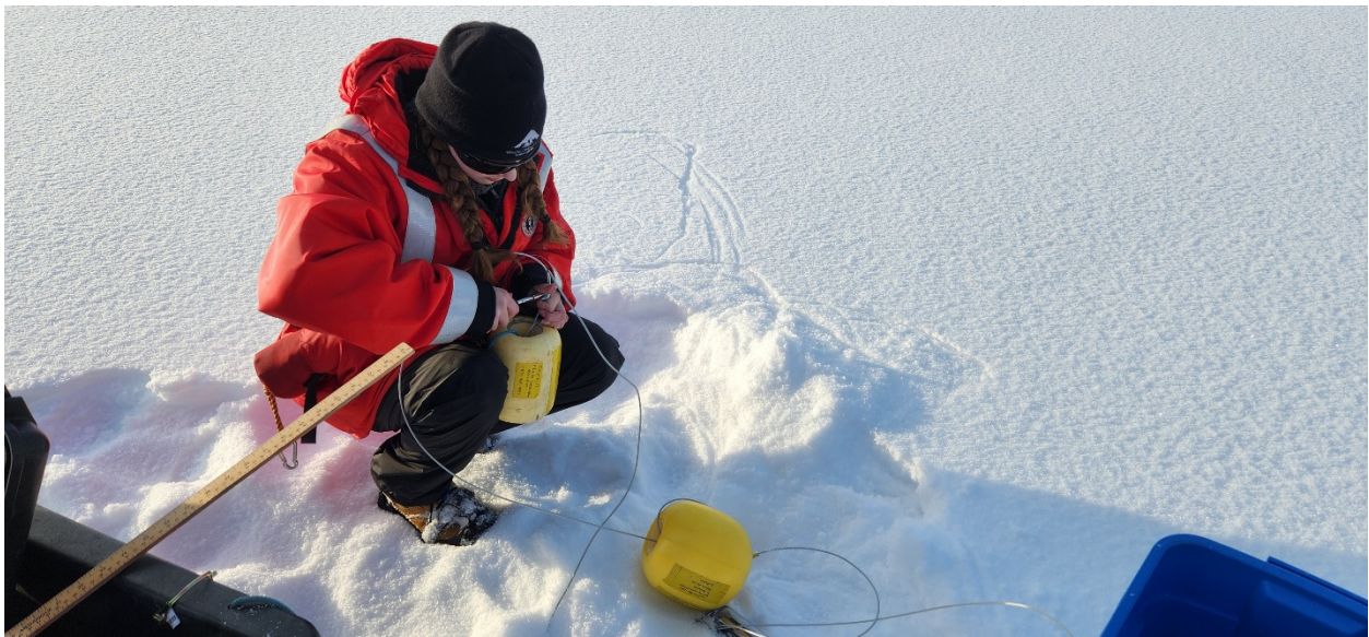
Photo 2. ACA staff rigging data loggers to a float line before being deployed in the pond. Photo: Troy Furukawa
