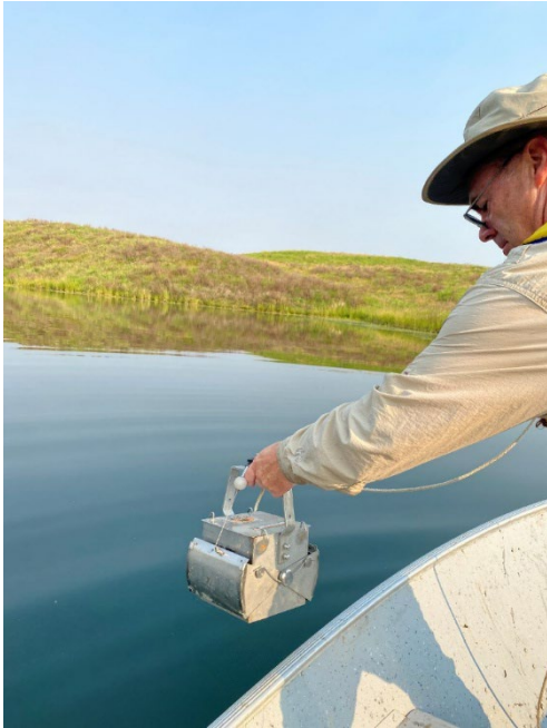
Photo 1. ACA staff member David Jackson preparing to deploy an Eckman dredge to quantify benthic invertebrate density as a forage base for stocked fish. Photo: Scott Seward
