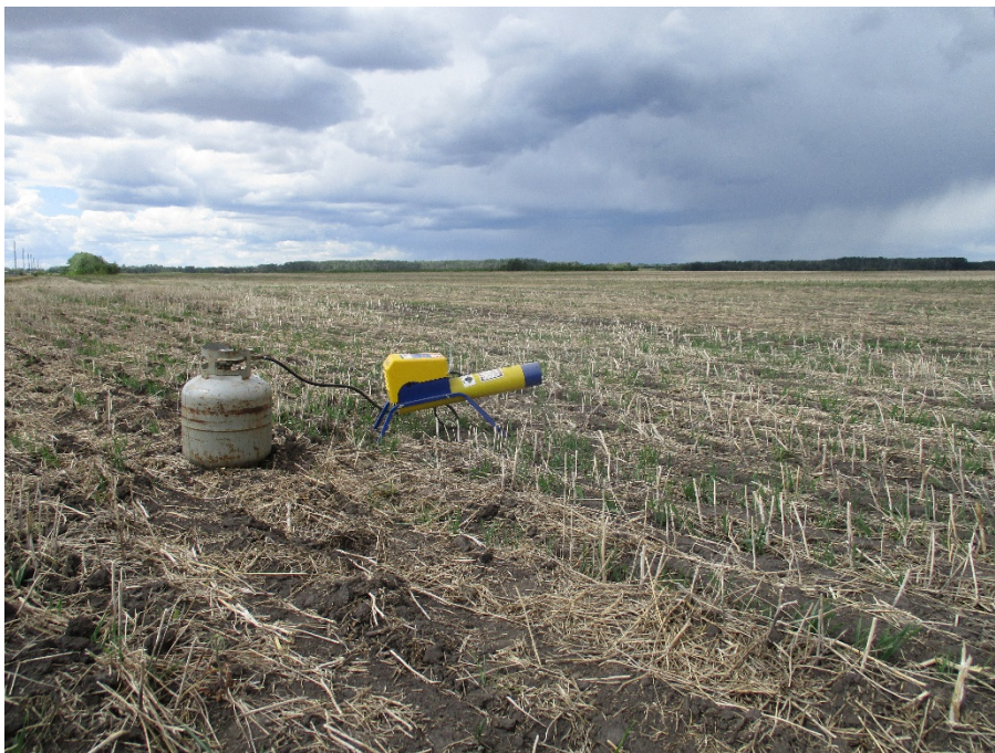
Propane scare cannon deployed in a stubble field. Photo: Ken Wright
