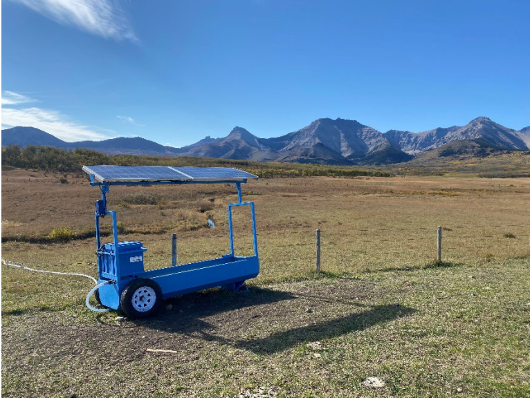
Photo 3. A solar-powered, portable watering unit reduces cattle pressure on sensitive riparian habitat on a ranch near Twin Butte in southwestern Alberta. Photo: Mike Verhage
