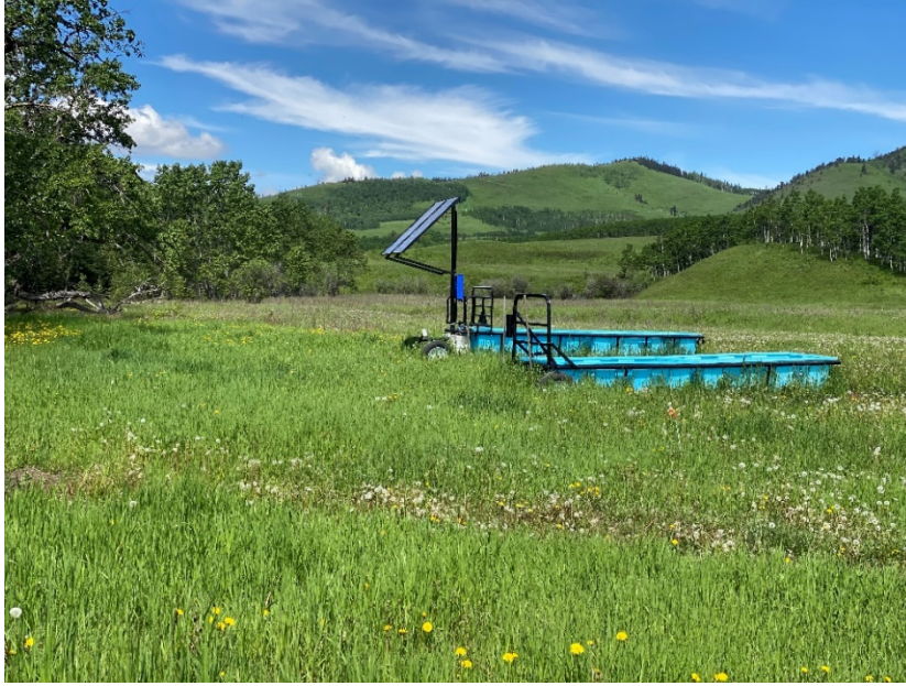
Photo 3. A solar-powered, double trough, portable watering unit provides clean water for cattle and reduces disturbance in the riparian area on a ranch near Chain Lakes in southwestern Alberta. Photo: Mike Verhage
