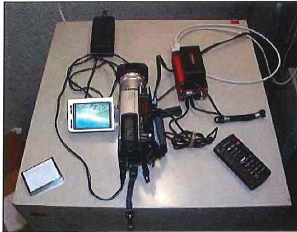
Figure 5. The Sony DCR-TRV 900 digital video camera and Red Hen Systems Global Positioning Systems mapping system used to record and geo-reference aerial videography.
